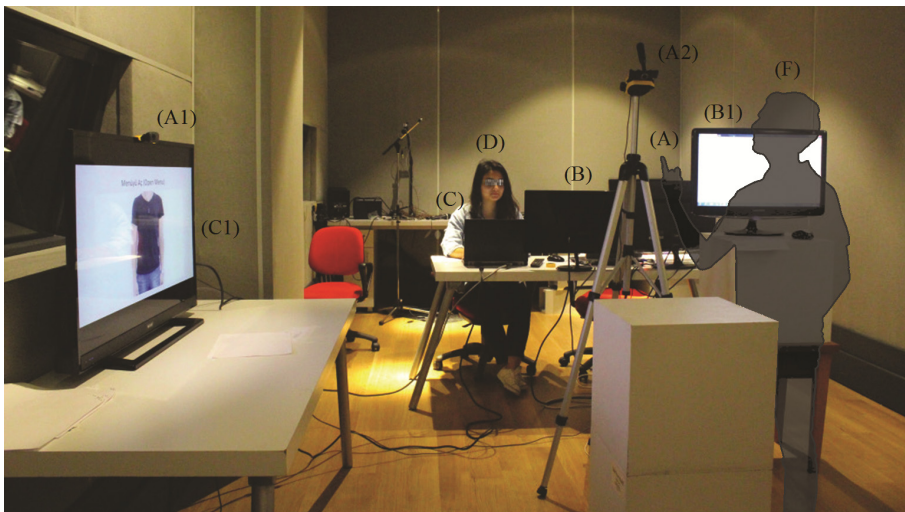
Fig. 1. The setting of the experiment: (A) Computer no. 1, (A1) Camera no. 1, (A2) Camera no. 2, (B) Computer no. 2, (B1) Survey screen, (C) Computer no. 3, (C1) LCD TV, (D) Wizard-of-oz, (F) Participant
