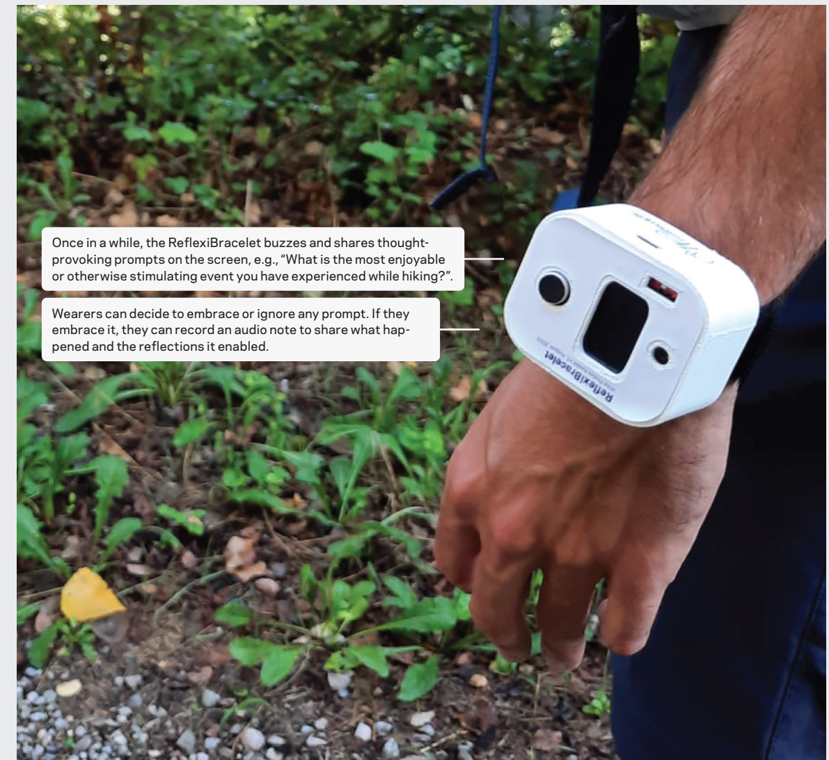
Fig. 6. Like the MemoCollar, the ReflexiBracelet enables seamless documentation through audio notes. Yet, this WP also sends thought-provoking questions to the wearer to encourage them to focus on specific aspects of their forestry experiences.
