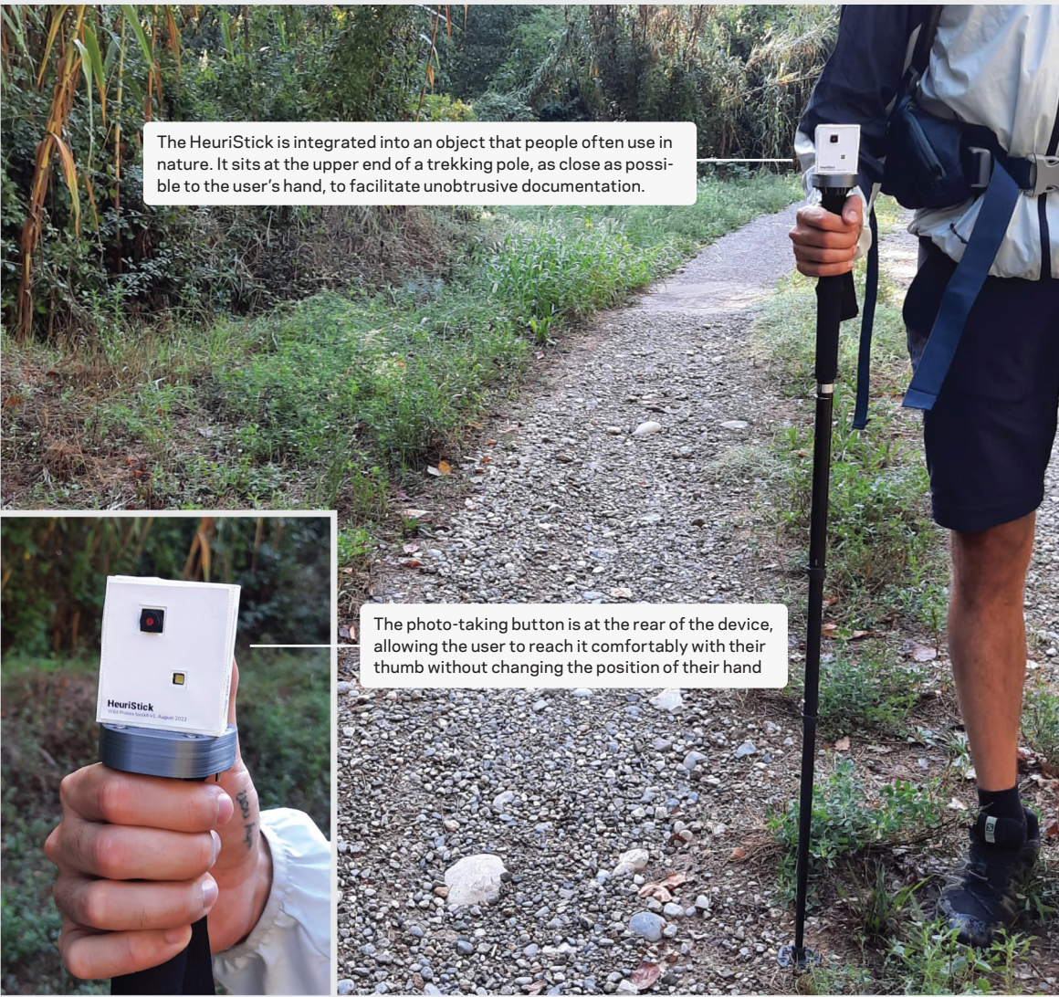
Fig. 2. The HeuriStick extends trekking poles by allowing users to rapidly document (on photo and video) spontaneous events.
