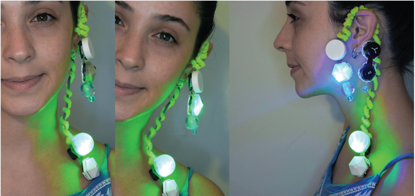
Figure 6: Left: IlluminEar in dim state, Middle: Changing colors with the head movement (green), Right: Side view of IlluminEar
